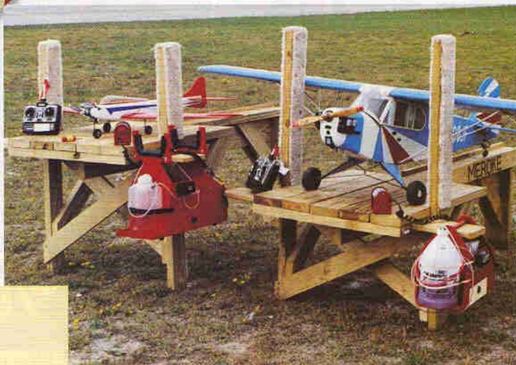
Standard bench on the left, with a Birdie 10 ready for starting; 1/4 Scale bench on the right, with a Piper Cub in readiness.
